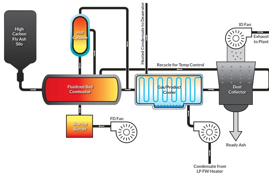
solely by the residual carbon within the fly ash, and the recovered heat is returned directly to the power plant. It may be used to beneficiate high-carbon fly ash either directly from the power plant or from fly ash that has been stored in landfills or ponds.
