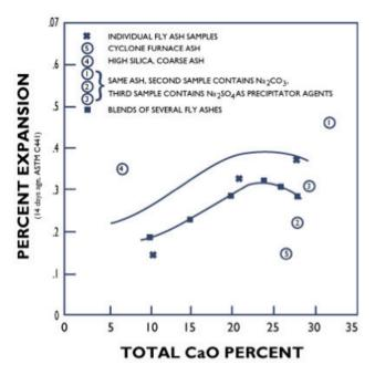
The decrease in alkali/silica reaction comes from the fact that Class F fly ash reacts chemically with and absorbs alkalis in the cement, thus making them unavailable for reaction later with the reactive aggregate.
