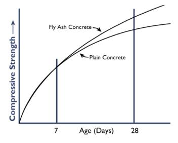
Fly ash concrete can be designed to achieve any level of strength obtainable by concrete containing only portland cement.
